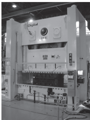
Photo 3 Over view of 3 000 kN servo press machine
